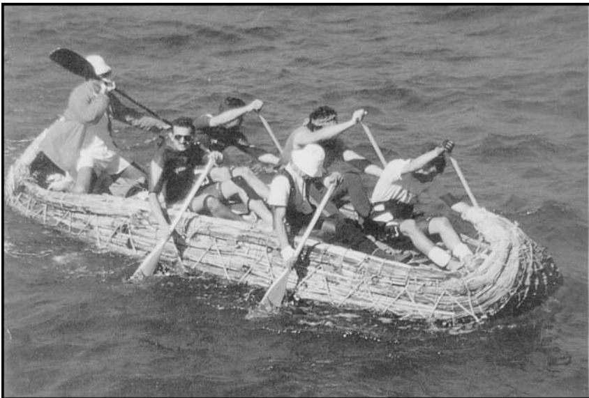
Fig. 5 Paddled experimental Papyrella reed boat. (photo: Henry Tzalas 1995)
